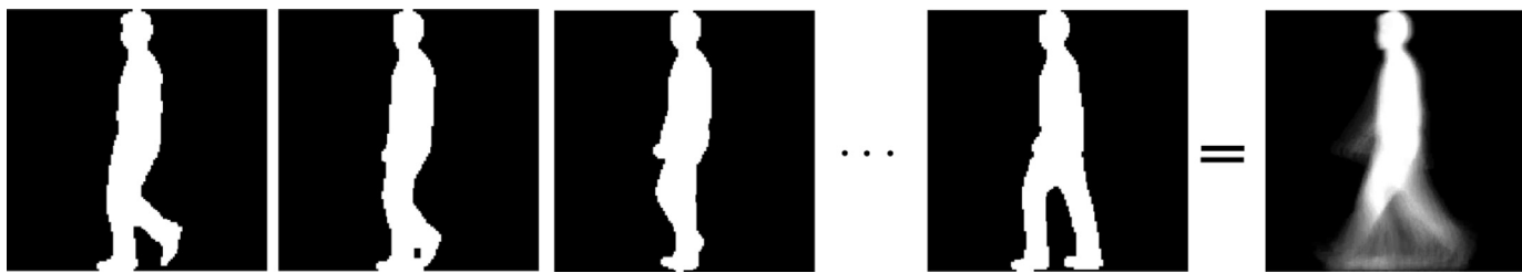
Fig. 1. A gait energy image (the right most one) is produced by averaging all the silhouettes (all the remaining images on the left) in one gait cycle.
