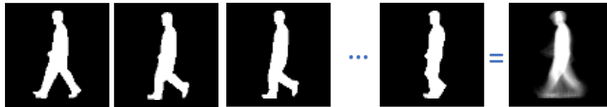
Figure 4: A gait energy image (GEI) [5] is obtained by aligning human silhouettes and averaging them.
